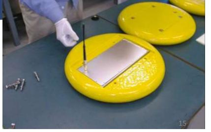
Standard : drifting buoy for oil spill tracking radius : 20 cm thickness : 5 cm weight : 4 kg material : expanded polyester
