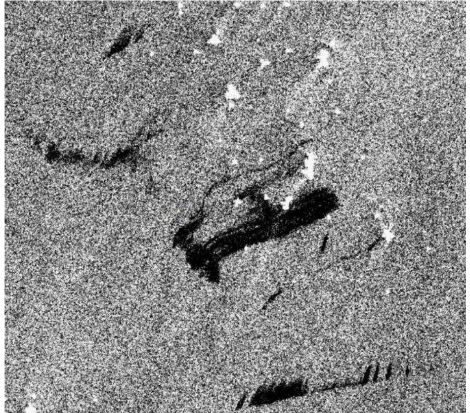
RADARSAT-2 image showing oil from offshore drilling platform. The oil appears as a dark tone and the offshore platforms appear as bright targets
