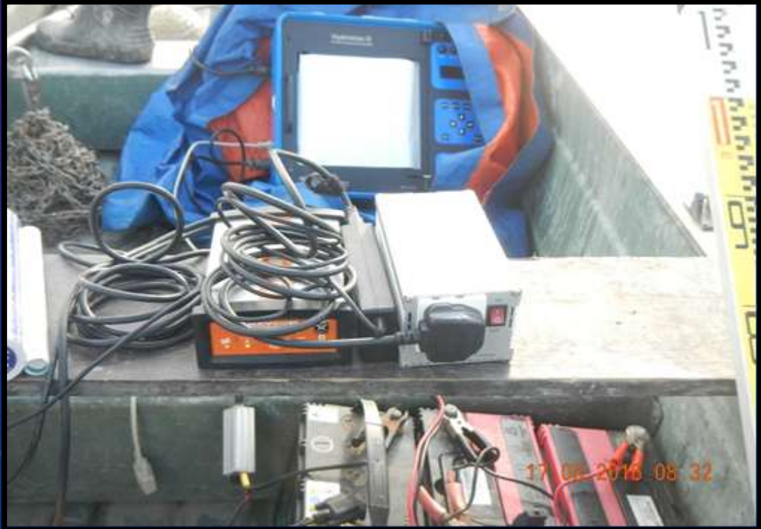
Bathymetric survey system on board
