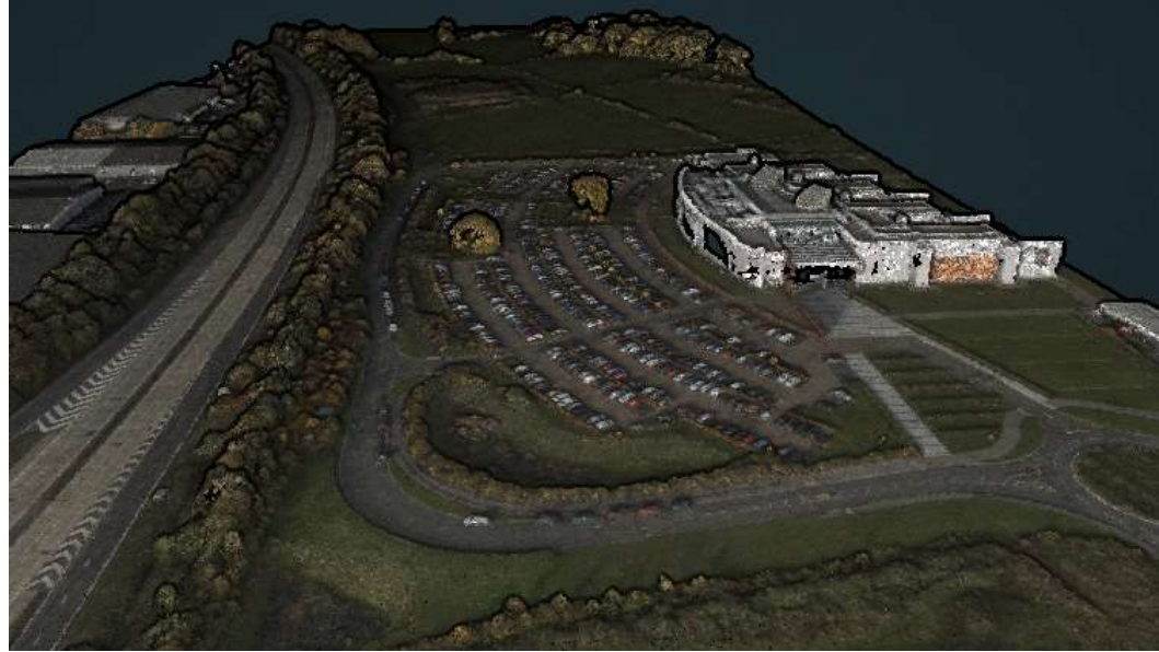
oblique camera point cloud
