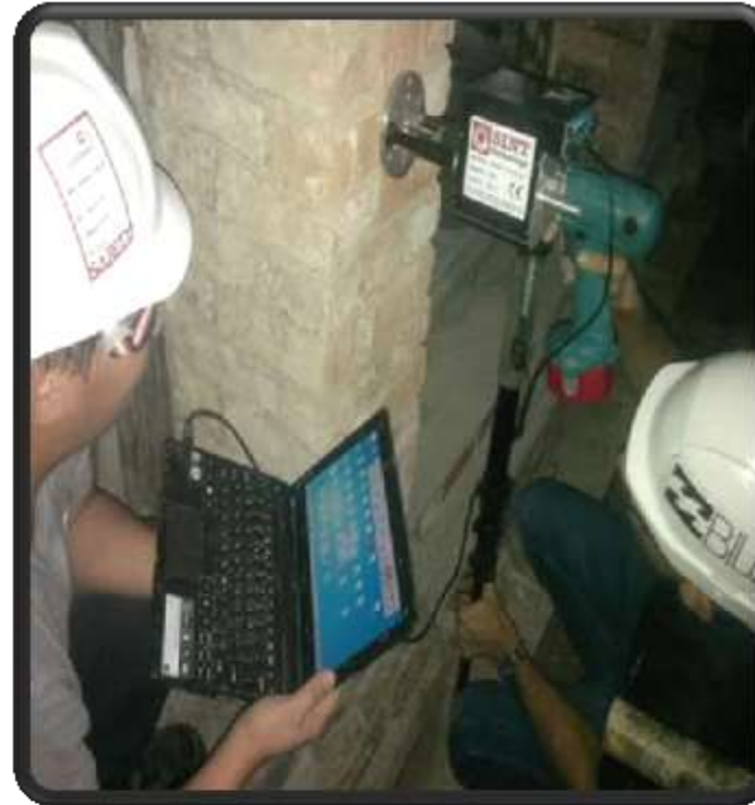
DRMS Cordless (Drilling Resistance Measurement System- measures the force needed for drilling and the position of the bit during drilling
