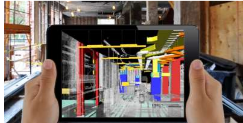
Superimposing beams and columns onto a real building
